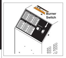
**STEP 4:** For hot water washing, turn the machine burner switch to the ON position. Adjust thermostat to desired temperature setting. (The burner will light automatically.)
